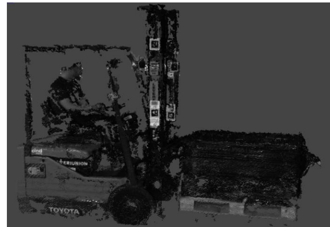
Point cloud illustrating plastic extending beyond one side of the load.
